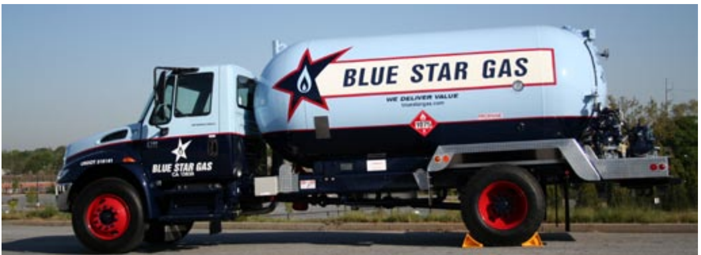
Blue Star Gas' brand new truck is an International 4300 chassis with 6-speed manual transmission and a DT466 in-line 6 cylinder diesel engine with 245 hp and 620 lb/ft of torque. An LCR-2 electronic register is tied into PDA and GPS systems.
